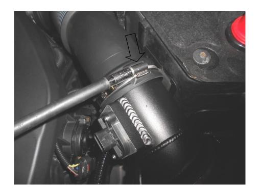
15. Reconnect the wiring to the MAF sensor.
