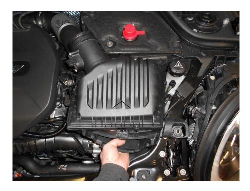
7. Using a T20 Torx driver undo the 2x screws and carefully remove the MAF sensor. Handle with care (Sensor shown is generic type and is for reference only).
