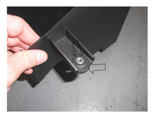
11. Carefully fit the airfilter tray in position and secure with the M6x20mm Allen bolt and 6mm penny washer.
